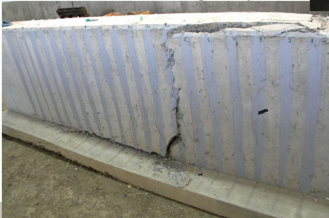
Tightly spaced CFRP-NSM
